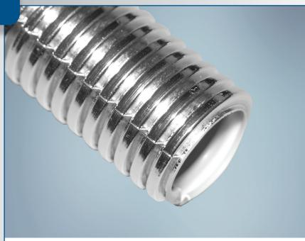
**ConvoShield**<sup>®</sup> **AL** is a reflective convolute sleeve designed to provide thermal protection for components in radiant heat environments. Composed of a high temperature nylon 4,6 polymer base substrate and a highly reflective coating, ConvoShield AL provides protection for wires, cables and hoses in applications that have radiant heat source temperatures as high as +538°C (+1000°F).
