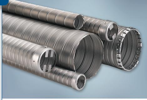
**ClevaFlex® Air Handling Ducts** are corrugated, stainless steel, flexible ducts with interlocked seams that are folded flat for airtightness, strength and flexibility.
