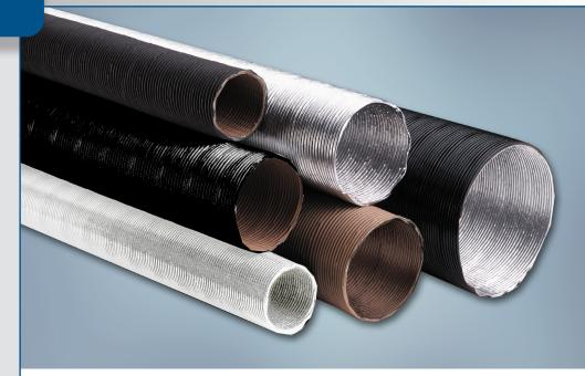
ClevaFlex® Air Handling Ducts are manufactured using multi-ply technology in which dies create convoluted flexible ducts that are permanently bonded with a thermosetting adhesive.
