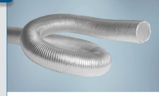
**Clevaflex® F-A** is a reflective corrugated tube designed to provide thermal protection for components in radiant heat environments. Its multi-ply construction of aluminum laminated fiberglass coupled with an aluminum foil exterior also allows for good insulation to components requiring stable temperatures for optimum performance efficiency.
