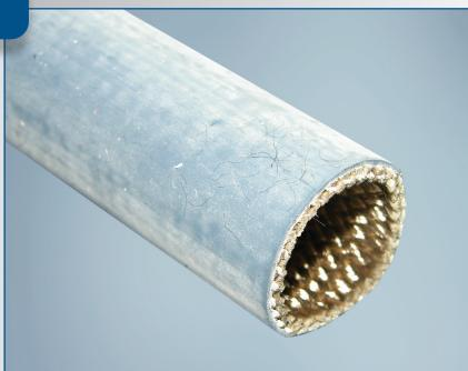
**Ben-Har<sup>™</sup> 1151-FRB Grade B** is a rugged, flame-retardant, silicone rubber coated sleeving that provides excellent cut-through and abrasion protection for wiring systems in applications with temperatures ranging from -70°C to +200°C. Because the specially formulated silicone rubber is extrusion coated over the non-combustible fiberglass braid, it results in a reinforced sleeving that is superior to ordinary dip-coated sleeving and unreinforced rubber or plastic tubing.
